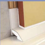
Each Sealux strip has a green tape applied to the inside face of the strip. Sealux-N silicone cannot bond to this tape after it cures. When joint movement occurs between the ledge and wall, the Sealux-N silicone simply releases off the green tape (under tension) and stretches to accommodate joint movement.
