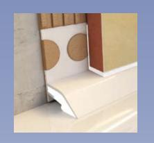
Each Sealux strip has a green tape applied to the inside face of the strip. Sealux-N silicone cannot bond to this tape after it cures. When joint movement occurs between the ledge and wall, the Sealux-N silicone simply releases off the green tape (under tension) and stretches to accommodate joint movement.
